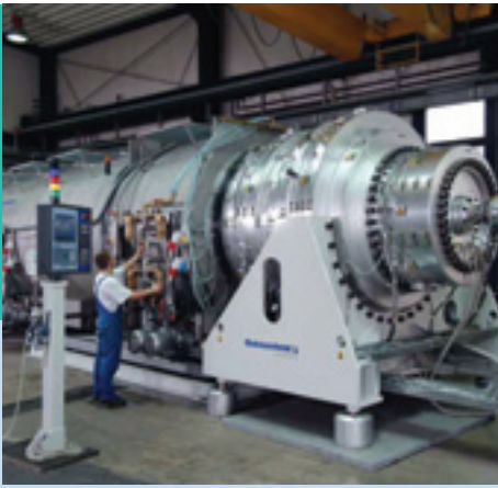
Picture 3: Details of the die head and calibration section
