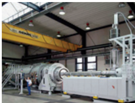
Picture 2: View showing the extruder barrel, die head and calibration section.
