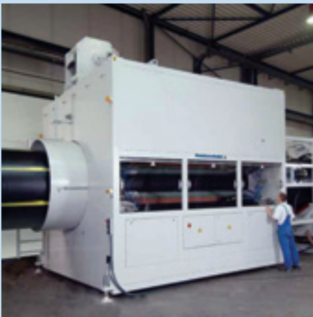
Picture 4: Haul off machine in operation
