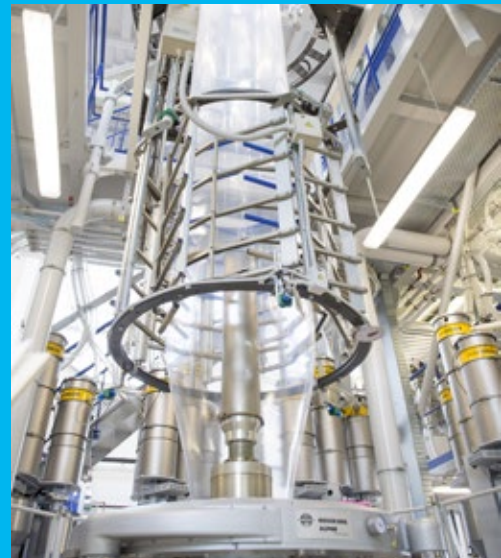
Multi-layer film made with Anteo™ FK1820 in skin layer processed in state of the art blown film line.
