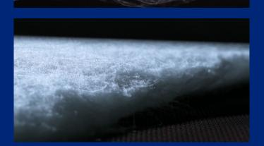
"Our RF5-BiCo technology enables producers to unlock the full potential of nonwovens. Matching BiCo with the right polymers helps attain properties — such as combined strength and fine fibers — which are not achievable with monocomponent fibres."
