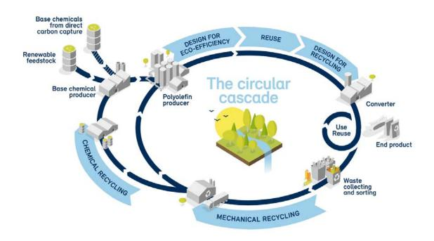
Illustration: Turing plastic back into plastic – By turning challenging and difficult to mechanically recycle plastic waste back into chemical feedstocks, chemical recycling is part of the solution to improve recycling rates while diverting plastic waste from landfill or incineration.
