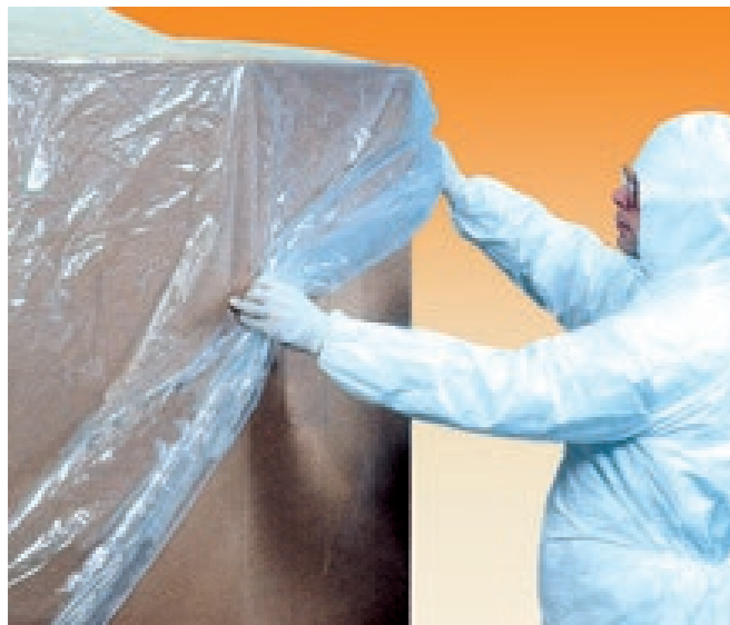
Step 3 Remove the lid and pull the dust protecting liner over the octabin.
