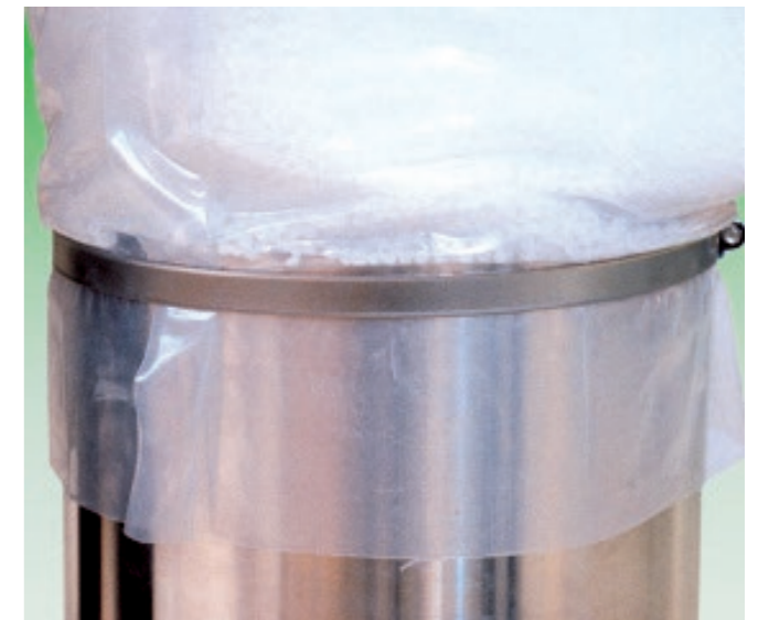
Step 8 Connect the hose to the filling pipe and open the strap for unloading.
