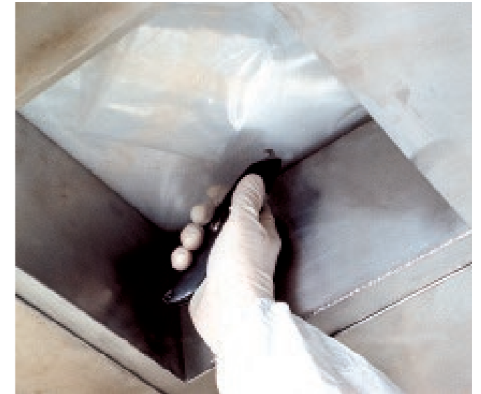
Step 6 Remove the hose protection. The covered octabin is now prepared for transfer to the unloading position in the clean room.
