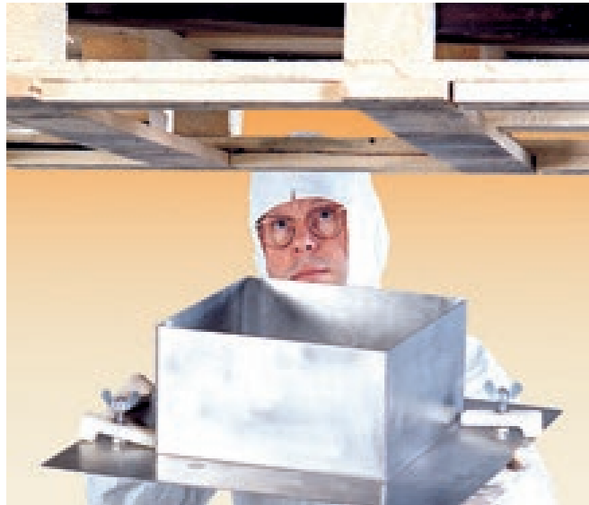
Step 1 Lift the octabin and insert the adapter in the bottom outlet frame of the pallet.
