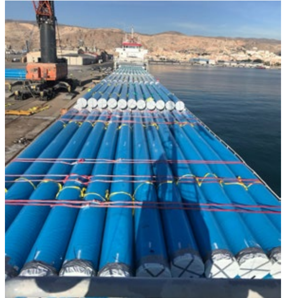
Figure 2: Pipes, coated by Noksel with a 3LPE coating system based on Borealis BorSafe ME3444, awaiting transport to the UK (photo ©Noksel Espana)
