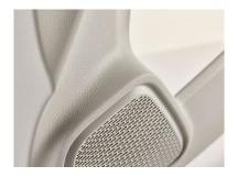
Borcycle™ EE1300SY: A 15% mineral-filled PP compound with 30% post-consumer recycled (PCR) content by weight. It combines excellent impact strength and stiffness with outstanding optics, scratch and mar resistance. Validated to OEM standards, it meets stringent emissions, fogging, and odor requirements. Available in standard dark to bright OEM colors.
