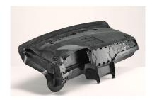
Fibremod™ GE277AI: A 20% chemically coupled, highflow fiber-reinforced PP compound for complex part geometries in standard and foam injection molding processes. Available with up to 50% renewable-based or chemically recycled polymer content by weight.
