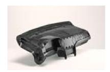
Borcycle™ GE2331SY: A 20% glass fiber reinforced PP compound with 40% post-consumer recycled content. Designed for injection molding of non-visible interior parts such as instrument panel or center console carriers, GE2331SY meets premium OEM requirements for emissions, fogging, and odor.
