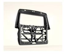
Fibremod™ GB416LF: A 40% long glass fiber reinforced PP offering high strength, excellent impact behavior, and premium aesthetics. Optimized for visible structural parts, it delivers scratch and mar resistance and low emission and fogging levels. Available with up to 50% renewable-based or chemically recycled content.
