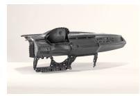
Instrument panel carrier in foamed PP long glass fiber 20% made from Fibremod GB601HP, a 60% long glass fiber reinforced PP compound diluted with EE002AE, a high impact strength elastomer modified PP resin.
