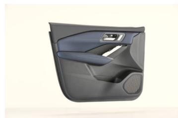
Daplen™ EG066AI is an elastomer modified PP intended for use in door panel and pillar trim applications. It offers an excellent balance between impact strength and stiffness at lowest possible material density and is available with 75% renewable-based or chemically recycled polymer content by weight.
