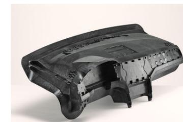
Fibremod™ GE277AI is a 20% chemically coupled, high flow fiber reinforced PP compound which allows for the production of complex part geometries in standard and foam injection molding processes.
