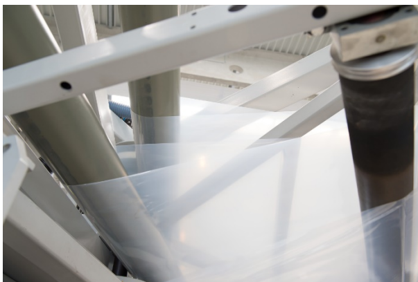
Photos: Anteo production at Borealis Innovation Headquarters' seven layer film machine
